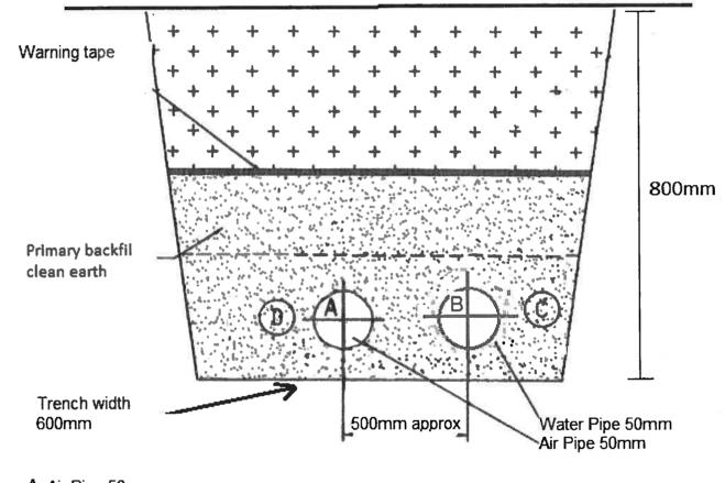
A-Air Pipe 50mm B-Water pipe 50mm C- Services
